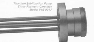
Titanium Sublimation Pumps offer an economical means of pumping chemically active (getterable) gases at high speeds. TSPs are highly efficient over a wide pressure range, from 10-2 Torr to below 10-11 Torr, and are compatible with other pumps that remove non-getterable gases.
