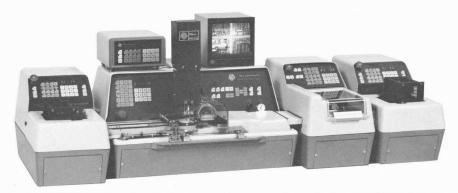
Model 2006 Wafer Cleaning Station is machine compatible with the MAI MODEL 3300 Wafer Dicing System shown above. Wafers mounted on Film Frame Carriers are unloaded from magazines in the Sender Module on the left. A continuous track automatically transports each wafer/frame through the dicing saw and MicroWash Cleaning Station, then into the magazine at the Receive Module on the right.
