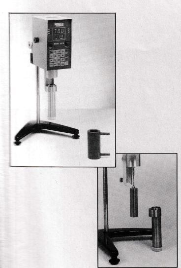
The Brookfield UL Adapter accessory has been developed for use with Brookfield Viscometers to allow accurate and reproducible viscosity measurements to be made on low viscosity materials. Newtonian and Non-Newtonian materials can be measured.
